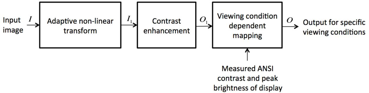
Figure 1. Block diagram of the proposed method
